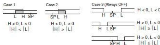
\*4. Set value: 5, Upper- and lower-limit with standby sequence For Upper- and Lower-Limit Alarm Described Above
