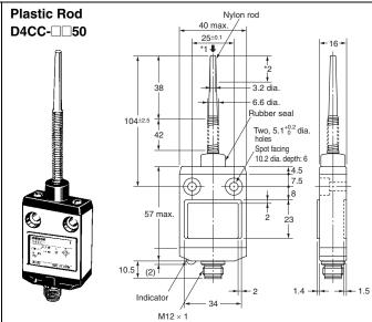
\*1. Operation is possible in any direction except parallel to the axis  $\Psi$ . \*2. The ideal range for operation is between the tip of the rod and 1/3 of the length of the actuator.
