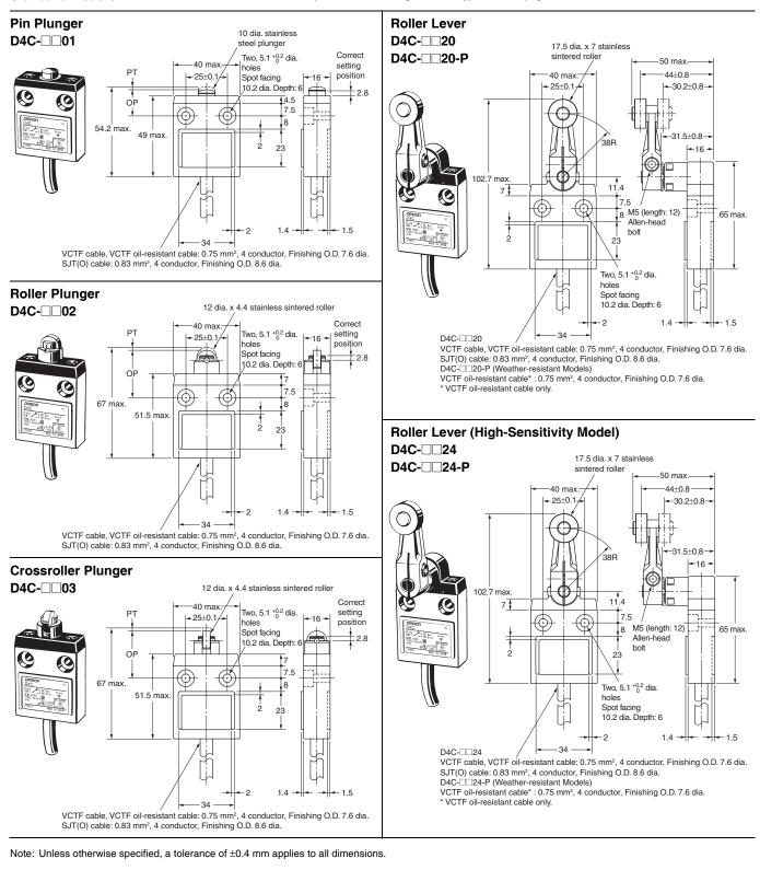
Model D4C-020 D4C-024 Operating D4C-001 D4C-002 D4C-003 D4C-020-F D4C-024-P characteristics Operating force OF max. 11.77 N 11.77 N 11.77 N 5.69 N 5.69 N min. Release force RF 4.41 N 4.41 N 4.41 N 1.47 N 1.47 N Pretravel PT max. 1.8 mm 1.8 mm 1.8 mm 25° 10°±3° Overtravel от min. 3 mm 3 mm 3 mm 40° 50° Movement Differential MD 0.2 mm 0.2 mm 3° 3° max. 0.2 mm Operating Position OP 15.7±1 mm 28.5±1 mm 28.5±1 mm ------
