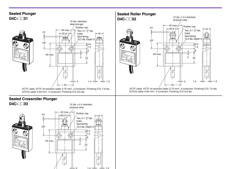
VCTF cable, VCTF oil-resistant cable: 0.75 mm², 4 conductor, Finishing O.D. 7.6 dia. SJT(O) cable: 0.83 mm², 4 conductor, Finishing O.D. 8.6 dia.
