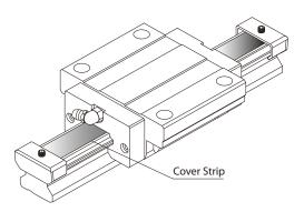
Note: When mounting the cover strip, the rail needs to be machined. The cover strip does not increase the height of rail.
