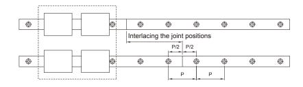
Fig.9 Staggering the joint position
