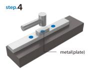
Continue pounding the cap until the cap is on the same plane with the top surface of rail.
