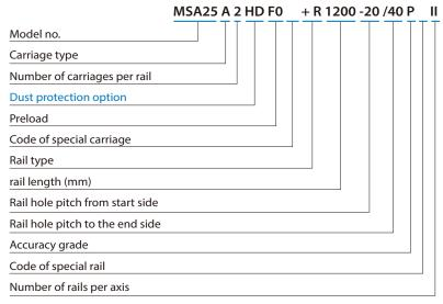
Note: Rail Model-MSA15, MSA20, MSA25, MSA30, MSA35, MSB15, MSB20(A type, E type, S type)
