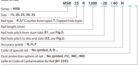
Note\*: U type rail is only applicable for MSB15 with M4 mounting hole.
