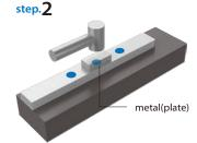
Put the plate on the cap, then pound it into the bolt of rail with rubber hammer vertically.
