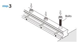
Check for correct bolt play and temporarily tighten all bolts.
