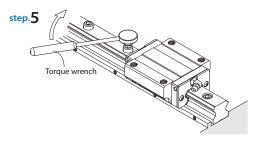
Tighten all bolts to the specified torque. The tightening sequence should start from the right side to the left side. By doing this, the original accuracy could be achieved.
