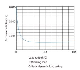
Relationship between working load and friction coefficient
