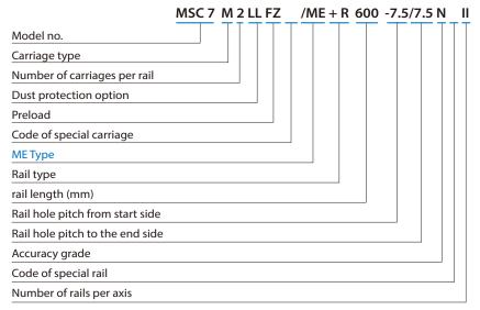
Note: Applicable specifications- MSC7M, MSC7LM, MSC9M, MSC9LM, MSC12M, MSC12LM, MSC15LM, MSC15LM, MSD12M, MSD12LM, MSD15M, MSD15LM.
