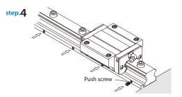
Tighten the push screw in sequence to ensure the rail close matching the reference side of bed.
