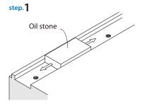
Prior to installation, the burrs, dirt, and rust preventive oil should be removed thoroughly.
