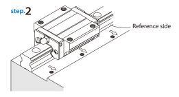
Gently place the linear guideway on the bed, and pushing it against the reference side of bed.
